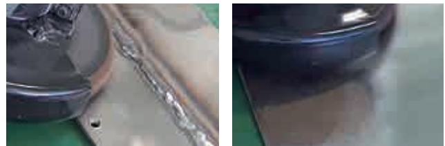
Removing blue weld discoloration Removing Rust
