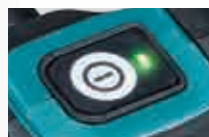
Main power switch with auto power-off function
