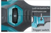
Setting up RPM at full up position of trigger is easy by a variable speed dial. Variable speed control by trigger enables to adjust RPM during operation.
